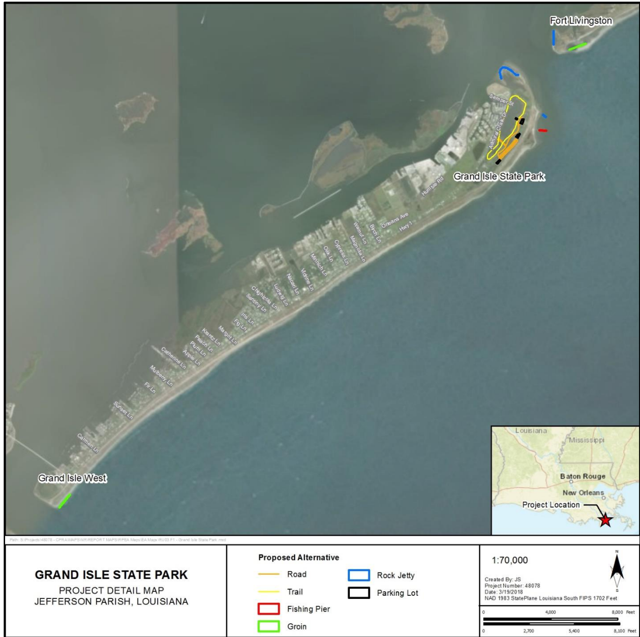
Figure 1. Location of elements within the Grand Isle State Park Improvements project location.
