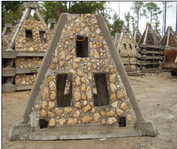
Figure 12-32. Example of a modular artificial reef unit that would likely be placed in deeper water.
