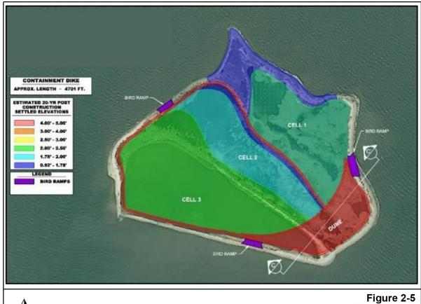
Figure 2-5 Design Alternative 4: Two-Phase Construction Queen Bess Island Restoration
