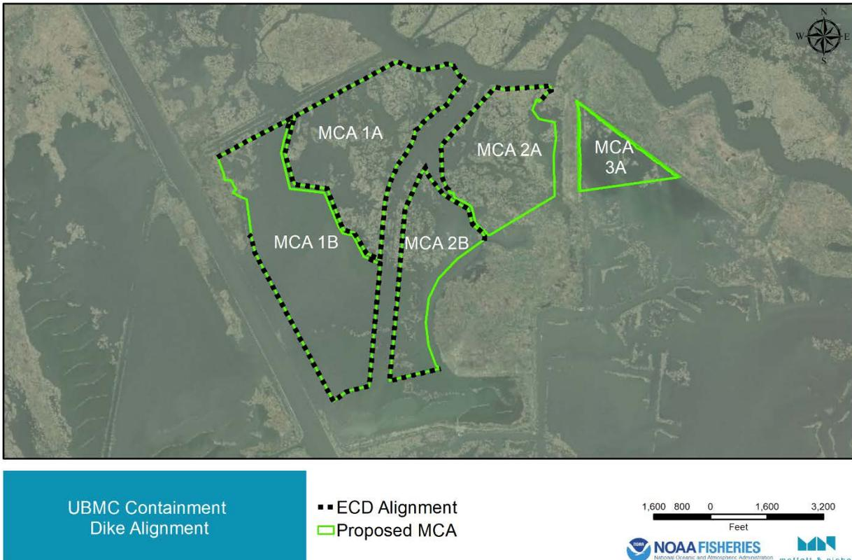
**FIGURE 3-4. Earthen containment dikes (ECDs) around MCAs.**
