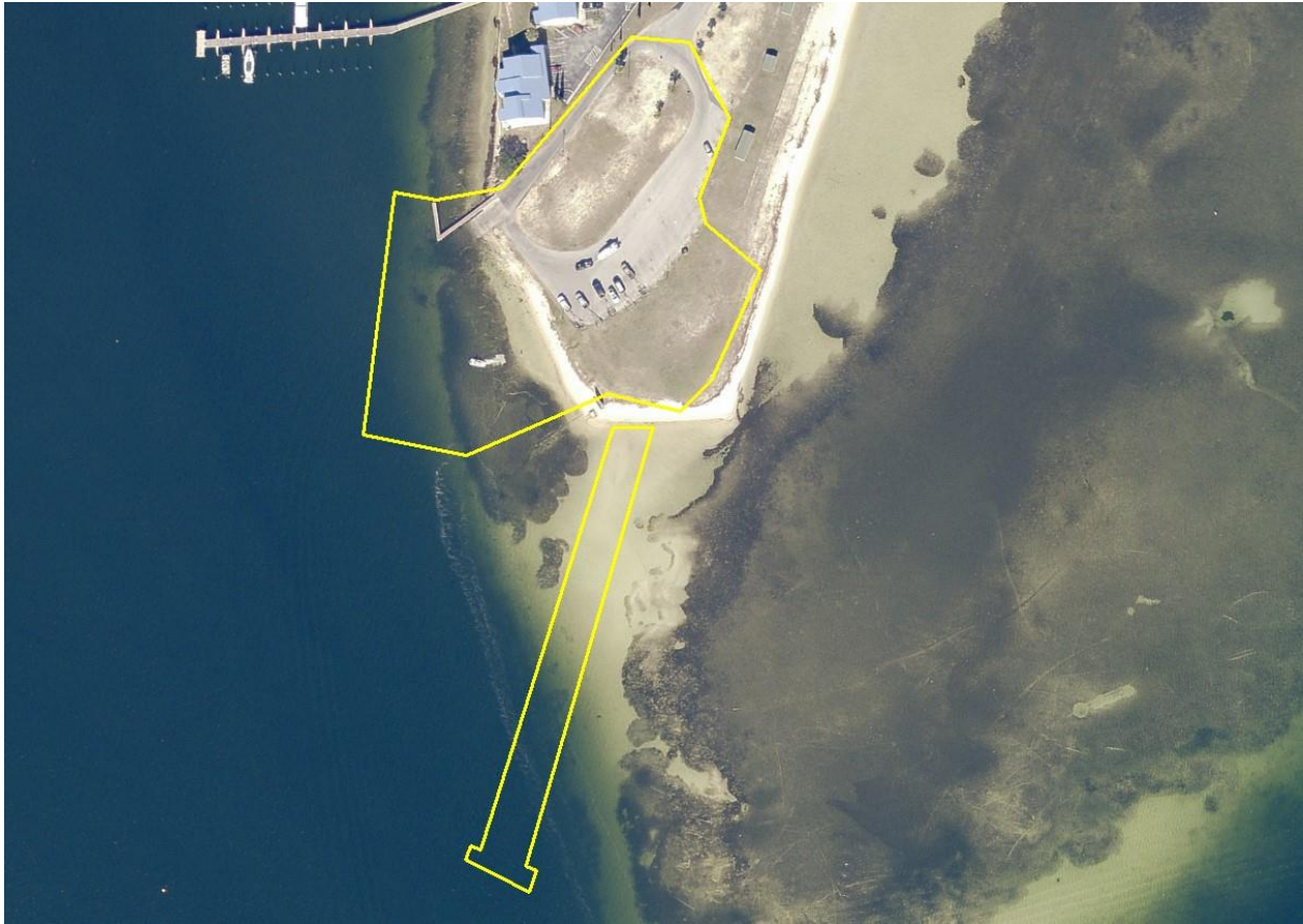
Figure 12-39). The boat ramp is approximately 50 feet long by 15 feet wide, and the existing L-shaped dock is approximately 100 feet long by 5 feet wide. The parking area currently contains approximately 12 parking spaces for vehicles and trailers.
