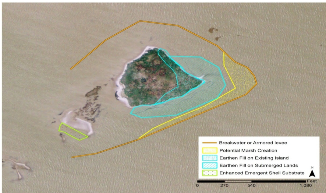
Figure 5-6. Conceptual drawing of the proposed Dressing Point Island restoration, illustrating the footprint of the breakwater/levee, fill, and emergent shell substrate
