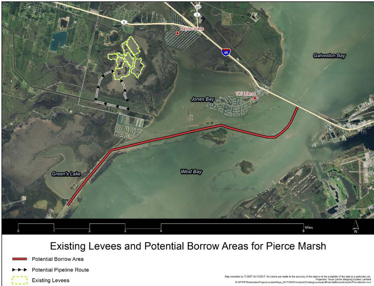
**Figure 3-8. Map showing the existing levees, potential borrow area, and potential pipeline route.**
