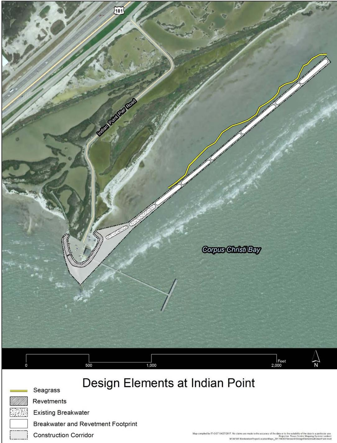
**Figure 3-12. Breakwater structure proposed for protection of the Indian Point shoreline.**
