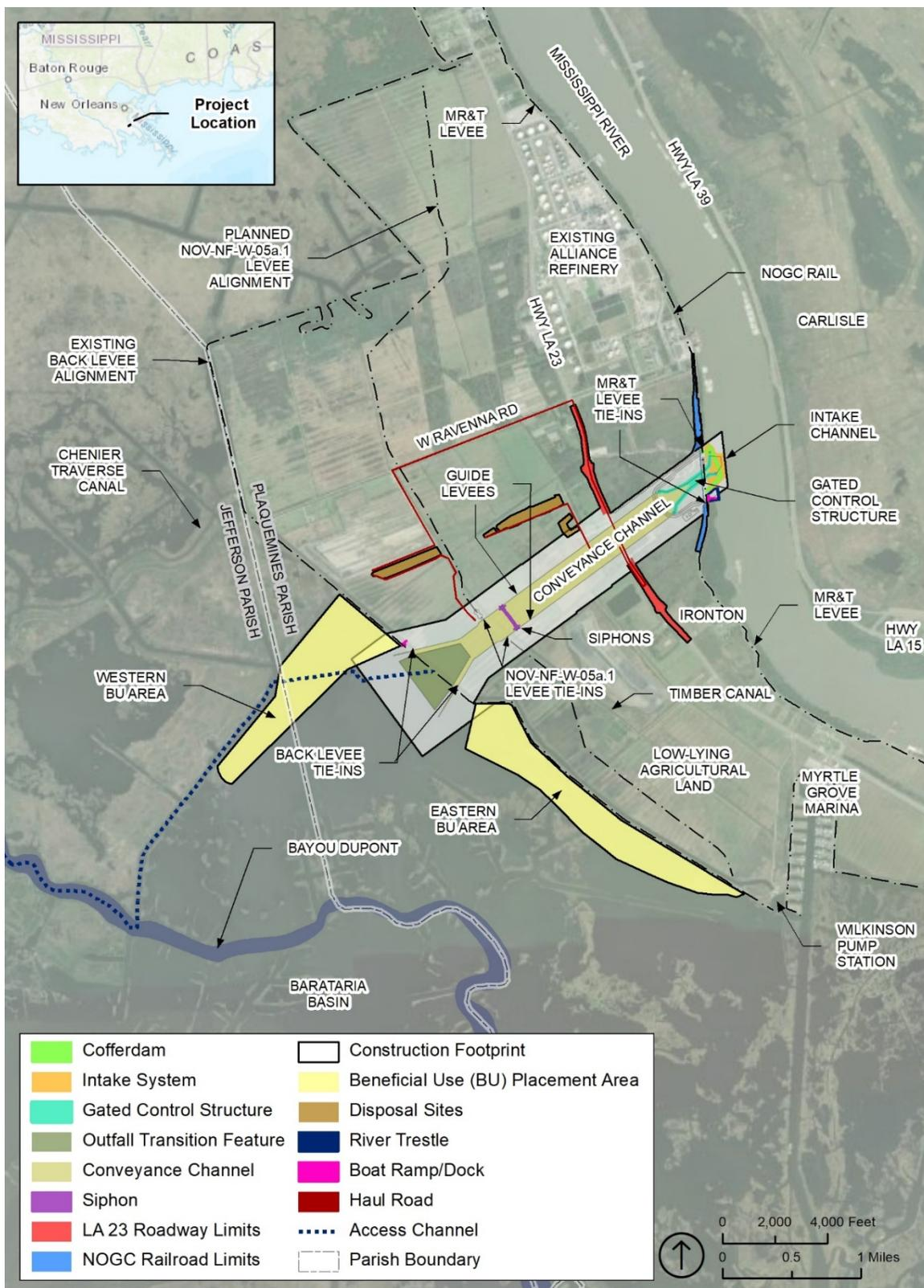
**Figure 1-2. Design Features and Construction Footprint of the Proposed MBSD Project and Its Alternatives.** NOGC = New Orleans and Gulf Coast Railway, NOV-NFL = New Orleans to Venice Non-Federal Levee.
